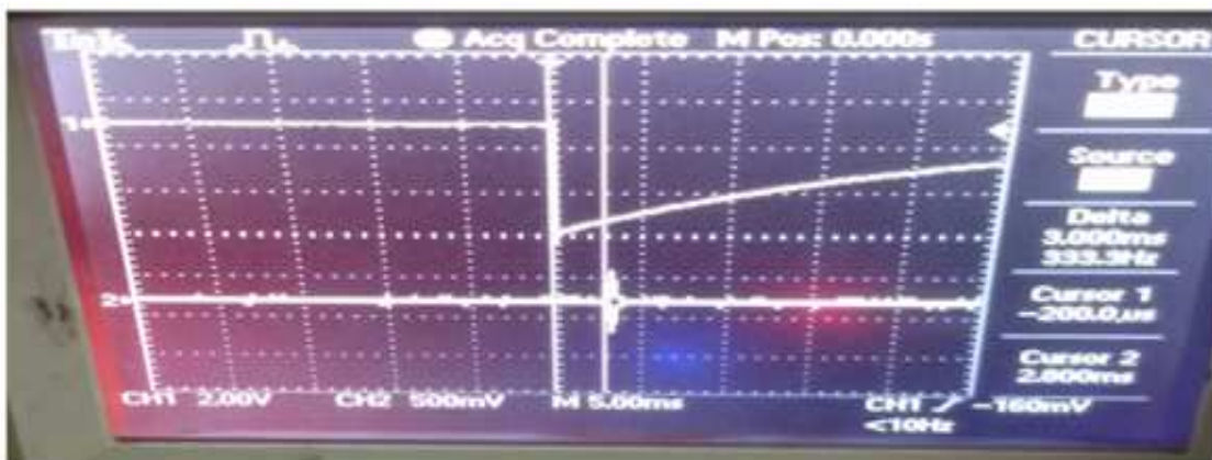
Figure 9b: DSO Output One Object Detected in the Steering Plane and Second Object not Detected Placed outside the Scanning Area
